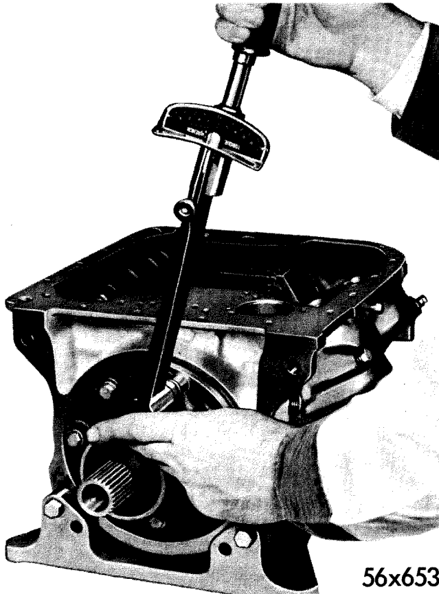
Figure 221—Tightening Front Oil Pump Housing Screws
