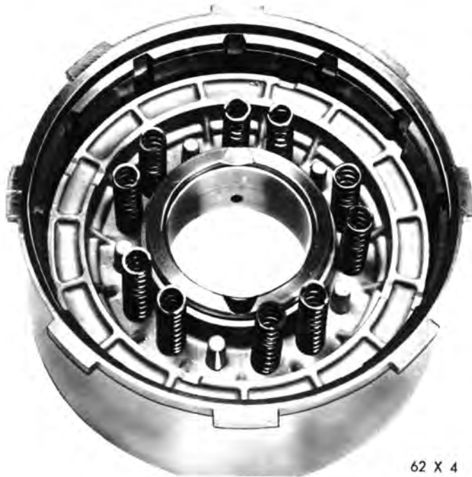
Fig. 95—Front Clutch Piston Return Springs —Location
