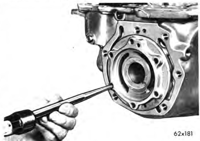
Fig. 108—Removing Overrunning Clutch Cam
