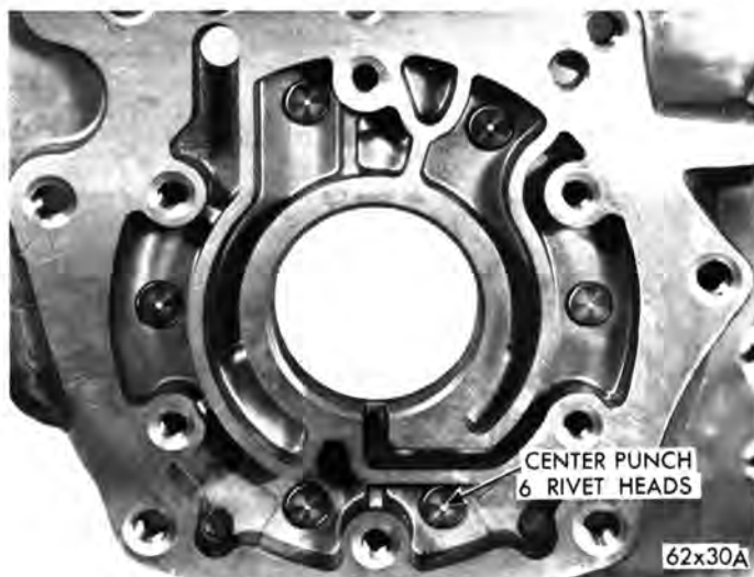
Fig. 106—Center Punch Rivet Heads
