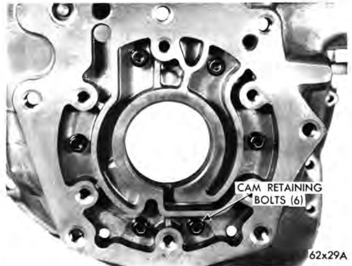
Fig. 107—Cam Retaining Bolts Installed
