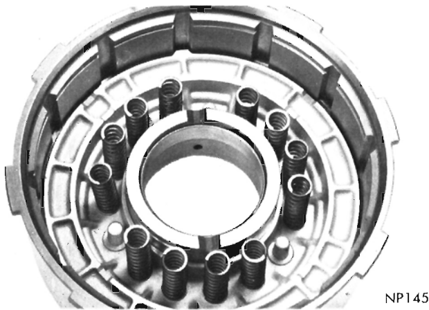
Fig. 74—Front Clutch Piston Return Spring Location (12 Springs)
