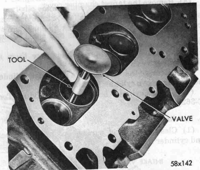
Fig. 20—Measuring Valve Stem Guide Clearance
