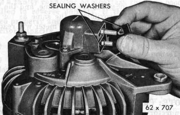
Fig. 30—Removing or Installing Sealing Washers
