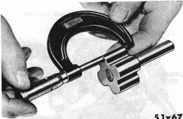
Fig. 65—Measuring the Inner Rotor Thickness
