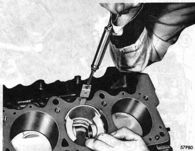
Fig. 14—Fitting Piston in Cylinder Bore
