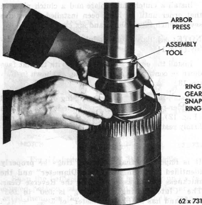
Fig. 23—Installing Ring Gear Snap Ring
