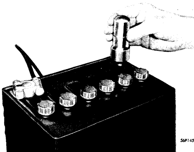
Fig. 2—Cleaning Outside of Battery Post
