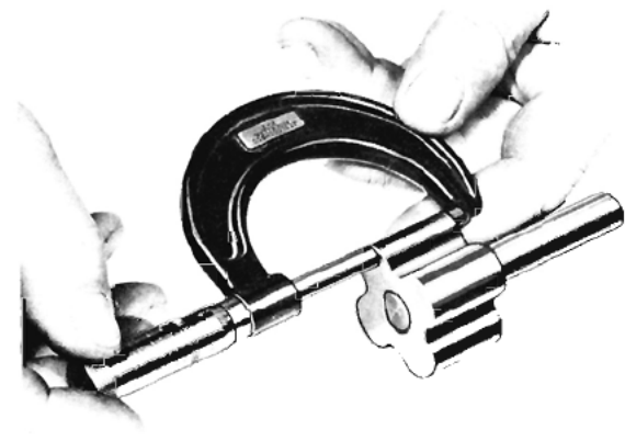
Fig. 125—Measuring Inner Rotor Thickness
