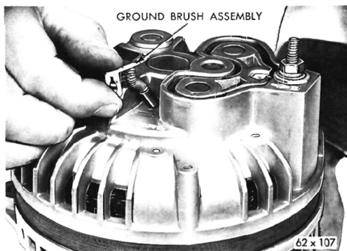
Fig. 16—Removing Or Installing Ground Brush
