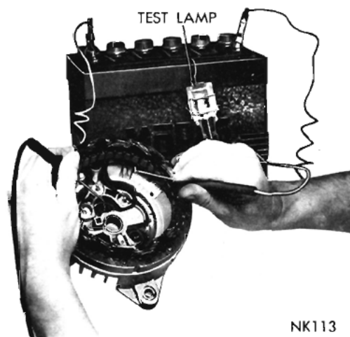
Fig. 23—Testing Stator Windings for Continuity
