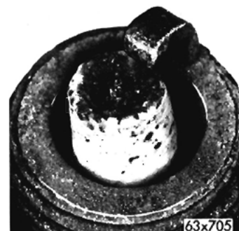
Fig. 11—Initial Pre-Ignition Damage
