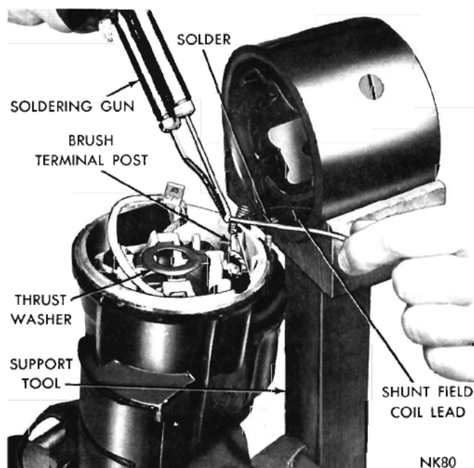
Fig. 24—Soldering the Shunt Coil Lead Wire
