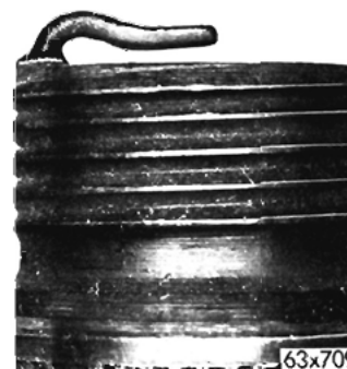
Fig. 15—Pressure Type Gap Tool Damage
