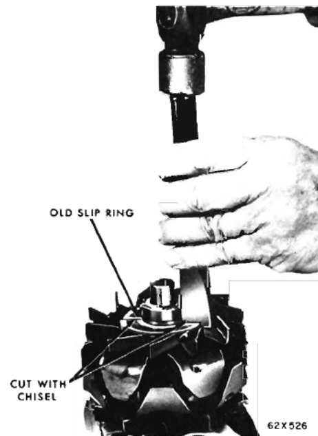
Fig. 31—Cutting the Old Slip Rings
