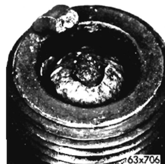
Fig. 12—Sustained Pre-Ignition Damage
