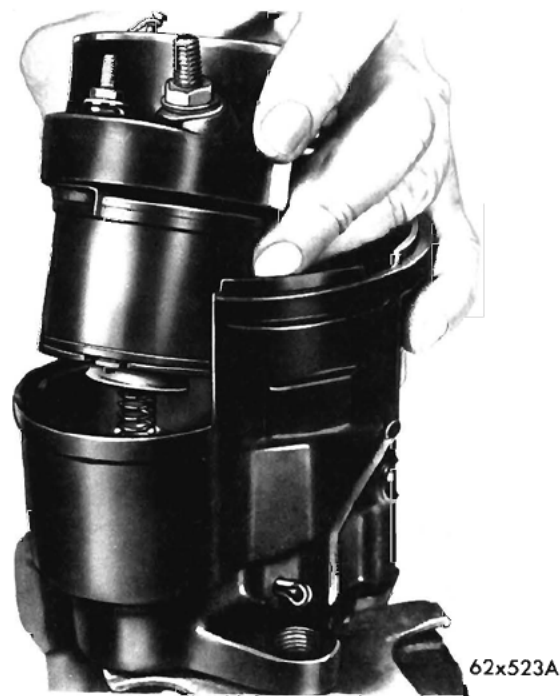
Fig. 23—Installing the Solenoid and Brush Holder into the Gear Housing
